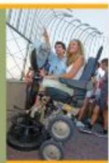
The wheels of the iBot wheelchair can lift a person to standing height.
